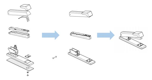
For the bottom subassembly, consisting of the **base**, **hanger**, **anvil**, and **clearing spring**, the parts are placed in an assembly jig that holds them in position to allow the **rivets** to be placed in the correct holes. Once the rivets are locked in place, a tool called an orbital riveter spins the hollow end of the rivet until it collapses outward and captures the parts together.
