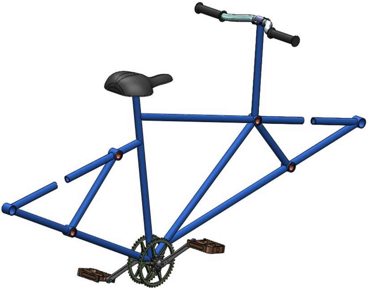
Figure 29 Body frame with some subassemblies
